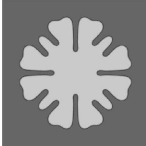
Fig. 1. Dendritic growth from the center at t=0.2 .
