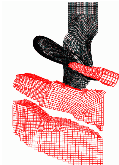
Fig. 5. Local embedded grid in the tip vortex region.
