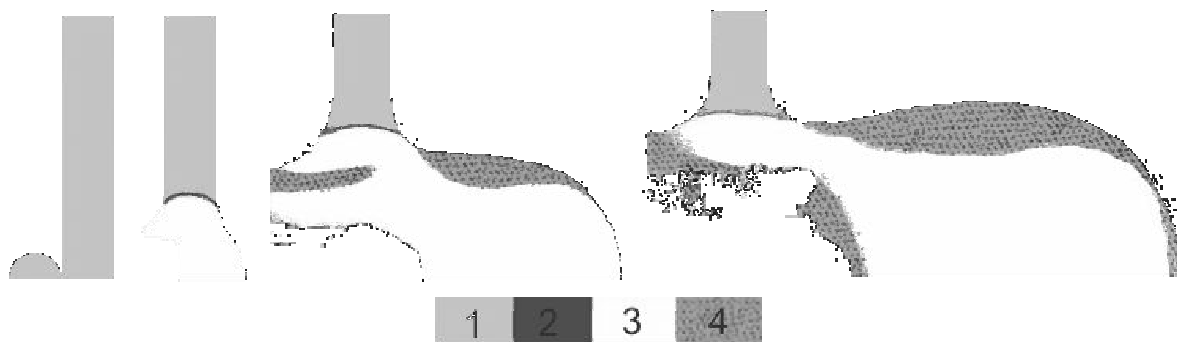
Fig. 3. Vertical cross-sections of density during hypervelocity impacts process. Regions marked 1,2,3,4 corresponds to solid, liquid, melted and evaporated material.
