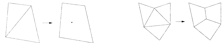
Figure 8.12: Left-hand side : the combination of two triangles gives one quad, right-hand side, the combination concerns four triangles and results in three quads.
